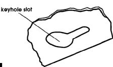
■ Lift range hood into final position and center. Mark on underside of cabinet the location for the four keyhole mounting slots. Set range hood aside on a protected surface.
